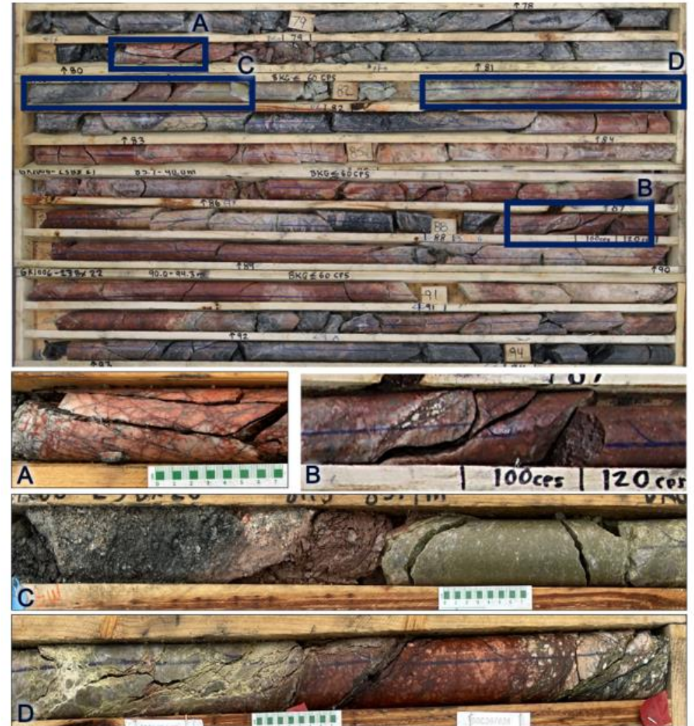
Figure 3: Photographs of alteration and deformation style intersected in a major faulted interval (shear zone) in drillhole GKI-006. A. Close-up of a hematized clast-supported crackle breccia with dark chlorite and hematite matrix. B. Close-up of strongly hematized fractured host rock with elevated CT-007-M scintillometer radiometry. Note the 3 cm-thick matrix-supported breccia exhibiting corroded clasts within a friable fine grained hematitic clay matrix. C. Close-up of a strongly altered cataclastic interval consisting of an incohesive gouge with dark grey to light grey clay matrix (left), an incohesive brick-red protobreccia (middle), and an indurated ultracataclasite zone with a sage green chloritic matrix (right). D. Close-up of continued strongly altered brecciated interval with brick red hematite noted overprinting the middle section of the photographed core and a later reactivation stage marked by a pale green-yellow clay matrix supporting chlorite-altered clasts.
